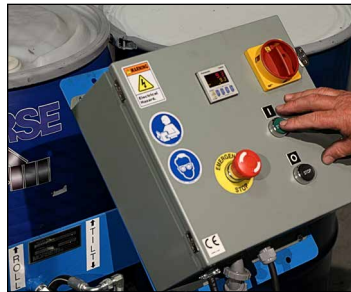
Push START button to activate power
