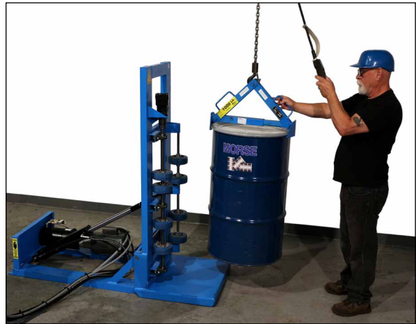
Load with your hoist or crane equipped with a Below-the-Hook Drum Lifter . Morse model 92 shown.
