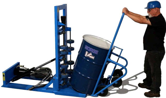
Load and unload drum with a drum truck such as Morse model 160 4-wheel drum truck shown here.
