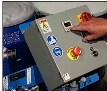
Set timer to Roll drum for desired time, from just a few seconds... up to 16 hours
