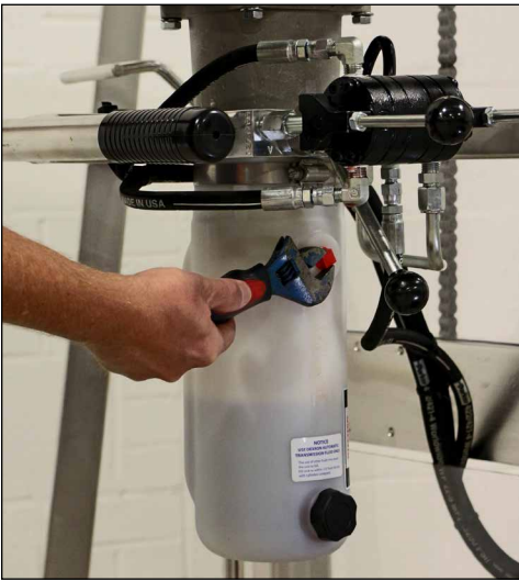
Remove RED shipping plug from the hydraulic reservoir
