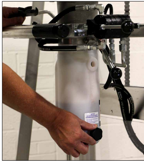
Remove BLACK breather from storage position
