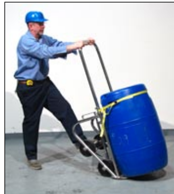
Strap assists in pulling your drum over onto the drum truck.
