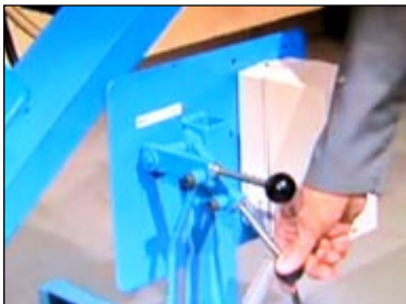
Lower the "TILT" lever to tilt the drum into horizontal position
