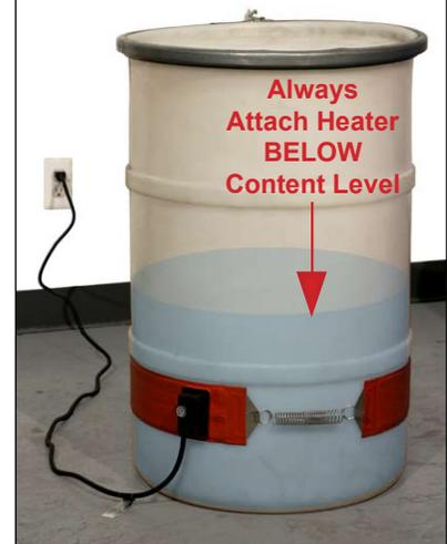
Drum heaters MUST be properly positioned BELOW the content level in the drum. Drum heater provides uniform heat over the 4" (10.16 cm) wide band around drum.
