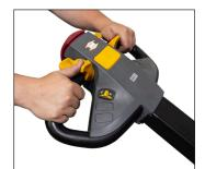
Familiar Controls for propulsion and steering. Raise and Lower Buttons incorporated in handle.
