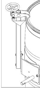
Figure 2.2 Plastic drum being lifted with part number 4560SS-PTop Rim Clamp Assembly installed.
